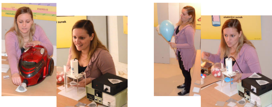
Fig. 3: Demonstration of radon progeny with filter and vacuum cleaner (left) and toy balloon (right)
